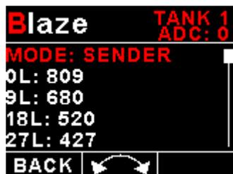
The fuel level sender needs to be calibrated before it can be used with this system. The calibration allows the system to learn the shape of your tank as well as any errors your fuel level sender or installation has.
