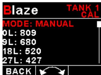
You may want to set individual calibration points manually. For example you may find that your fuel level is over reading at a specific fuel level. Correcting the tank level reading for this area can be simply done by adjusting the calibration point. You can do this by moving the float level with your hands to the desired position and then performing the calibration as outlined above, or you can use the manual option.
