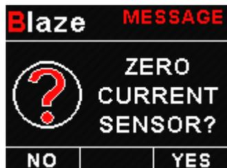
Select this function to indicate to the FLIGHT-3 that zero current is flowing through the MGL Avionics Closed Loop Current sensor. This is best done with the MGL Closed Loop Current sensor disconnected from the main current supplying conductor.
