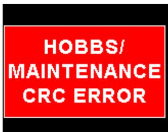
Hobbs / Maintenance Timer CRC error. Try entering new values for the Hobbs meter and Maintenance timer and see if the error message disappears. If the error message still persists then it could possibly be a non-volatile memory failure in which case the instrument will then have to be returned to the factory.
