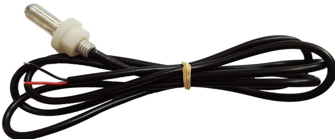
Connect the OAT probe red wire to the FLIGHT-3 analog input and the black or green wire to ground.
