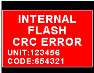
Internal flash CRC error. The instrument does a firmware check on the program when power is applied to the instrument . If the program is corrupt in any way then the internal flash CRC error will be displayed. Reload the instruments firmware and load default settings. If the error message still persists then it could possibly be an internal flash memory failure in which case the instrument will then have to be returned to the factory.
