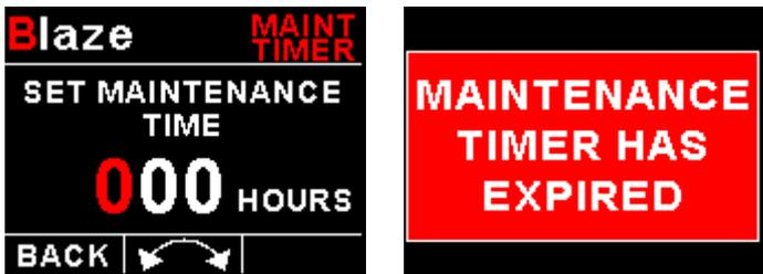
This function allows you to set an engine maintenance timer. This timer is set in engine hours and it will count down to zero when the engine RPM is greater than the "HOBBS RPM". A good use for this function is to set the hours until your next spark plug change or engine inspection. Use the rotary control to change the value.
