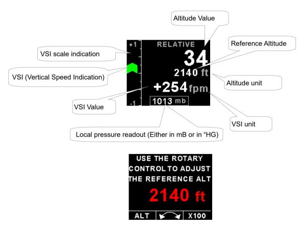
Press the F2/Down button during the Relative Altitude display to access the altitude reference screen. Press the F1/UP key to set the reference altitude to the current altitude or use the rotary control to adjust the reference altitude. Press the F2/Down key to change the increment / decrement unit to 10 or 100. Press the rotary control to exit and save.
