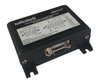
The CNV-ALT accepts RS232 serial data from a compatible MGL Avionics instrument and produces parallel Gillham codes in a format compatible with mode C transponders. The ALT-6 serial protocol must be set to MGL Avionics.
