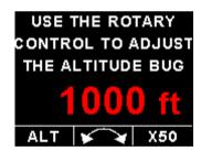
Press the F2/Down button during the altitude "TAPE" display to access the altitude bug setting screen. Press the F1/UP key to set the altitude bug to the current altitude or use the rotary control to adjust the altitude bug. Press the F2/Down key to change the increment / decrement unit to 50 or 500. Press the rotary control to exit and save.
