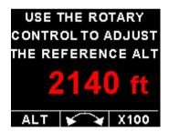
Press the F2/Down button during the Deviation Altitude display to access the altitude reference screen. Press the F1/UP key to set the reference altitude to the current altitude or use the rotary control to adjust the reference altitude. Press the F2/Down key to change the increment / decrement unit to 10 or 100. Press the rotary control to exit and save.
