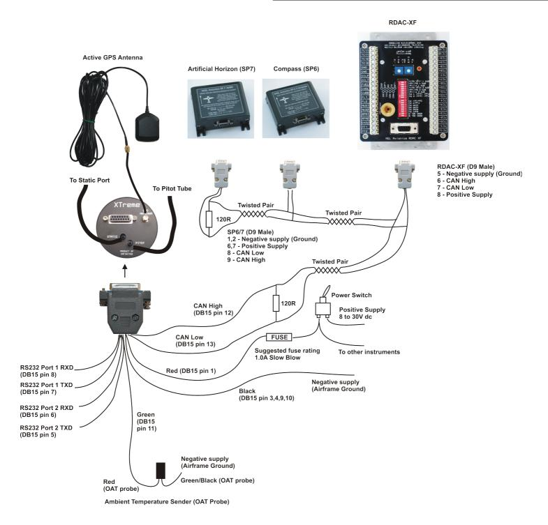
The use of an external 1A fuse is recommended. Connect the supply terminals to your aircrafts power supply. The XTreme can be used on both 12V and 24V without the use of any pre-regulators. Ensure that the supply voltage will not drop below 8V during operation as this may result in incorrect readings.
