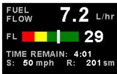
**3.1.4.2 Dual fuel flow and calculated tank levels (dual tank)**
