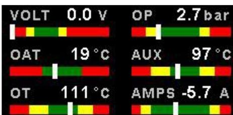
This section displays the supply voltage, OAT, oil temperature, oil pressure, as well as the 2 auxiliary analog channels. The oil temperature/pressure as well as the 2 auxiliary analog channels can be configured in the "EMS SETUP" menu.
