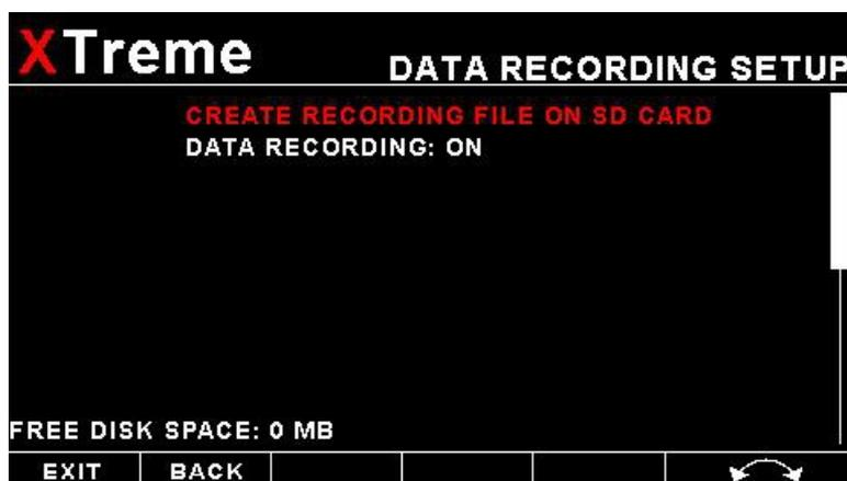
The XTreme-EMS has the ability to act as a black box recorder recording flight data directly onto an inserted SD card for later playback and investigation using the MGL Avionics Black Box viewer program. See the Black box viewer documents for further information. The Black box viewer can also convert the data into other file formats such as:
