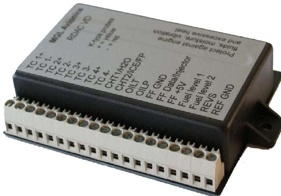
The RDAC model VD is an integrated, microprocessor controlled engine monitoring subsystem. It is intended for installation close to the engine, inside the engine compartment thereby eliminating the need for long probe and sender wires. **If using the RDAC-VD then the RDAC protocol setting in the miscellaneous section must be set to normal.**
