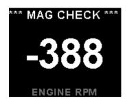
Press the F2/Down button once you have reached your normal run-up RPM. The display will show the RPM deviation from when the magneto function was activated. Any RPM drops will be displayed as a negative RPM value, a positive reading indicates an increase in RPM.
