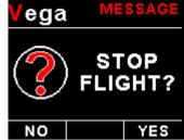
Press the F1/Up button during the normal display mode to manually start/stop a flight. This key is only active if the ASV-1 is setup to select the manual flight option under the "TIMERS" setup menu.
