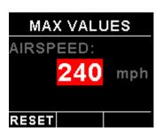
This display can be accessed by pressing the F2/Down button during the normal display mode. Press the F1/Up button when the max values display is showing to reset the maximum values to the current airspeed.
