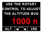
Press the F1/Up button during the altitude "TAPE" display to access the altitude bug setting screen. Press the F1/Up key to set the altitude bug to the current altitude or use the rotary control to adjust the altitude bug. Press the F2/Down key to change the increment / decrement unit to 50 or 500. Press the rotary control to exit and save.
