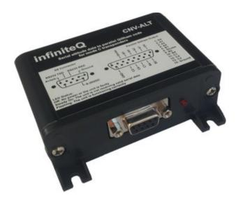
The CNV-ALT accepts RS232 serial data from a compatible MGL Avionics instrument and produces parallel Gillham codes in a format compatible with mode C transponders. The ASV-1 serial protocol must be set to MGL Avionics.
