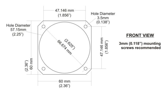
**NOTE:** 57.15mm (2.25") is a standard cutout, but due to manufacturing tolerances, 58mm (2.28") is found to be more desirable.
