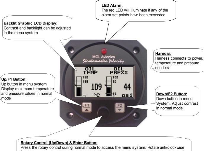
Press the rotary control during normal mode to access the menu system. Rotate anti/clockwise for up/down menu scrolling. During normal mode rotating the rotary control will toggle between the temperature and pressure display (only if Single display mode is selected).
