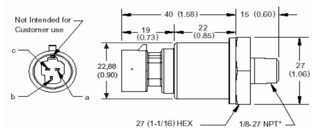
The sensor cable is approximately 3m long and has 3 leads. The black lead is not to be connected and has no function. The Red lead from the sensor has to be connected to the positive bus via a fuse or circuit breaker. The white lead (Output signal) has to be connected directly to the TP-2 Yellow wire (Pin 8).
