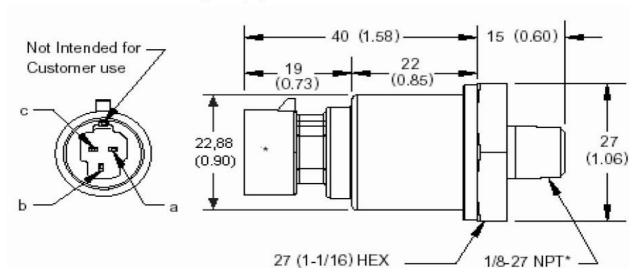
The sensor cable is approximately 3m long and has 3 leads. The black lead is not to be connected and has no function. The Red lead from the sensor has to be connected to the positive bus via a fuse or circuit breaker. The white lead (Output signal) has to be connected directly to the TP-1 Yellow wire (Pin 8).
