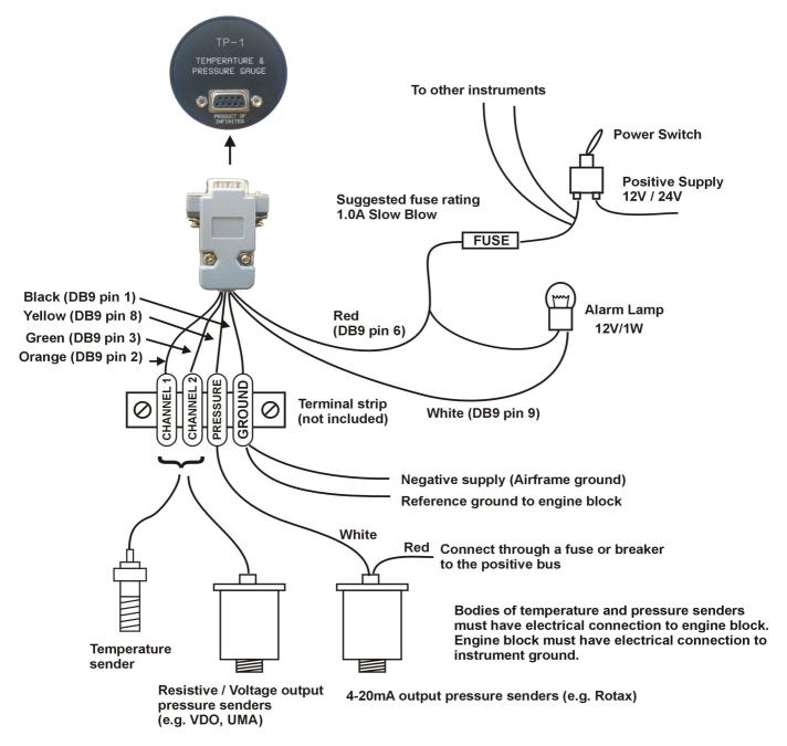
The use of an external 1A fuse is recommended. Connect the supply terminals to your aircrafts power supply. The TP-1 can be used on both 12V and 24V without the use of any pre-regulators. Ensure that the supply voltage will not drop below 8V during operation as this may result in incorrect voltage and or current readings.
