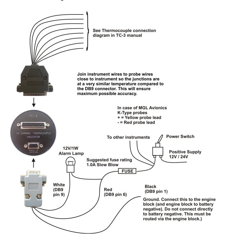
The use of an external 1A fuse is recommended. Connect the supply terminals to your aircrafts power supply. The TC-3 can be used on both 12V and 24V without the use of any pre-regulators. Ensure that the supply voltage will not drop below 8V during operation as this may result in incorrect readings.
