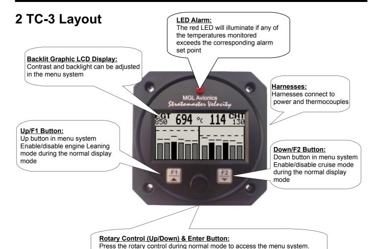
Rotate anti/clockwise for up/down menu scrolling. During normal mode rotating the rotary anti/clockwise will display the maximum values recorded.
