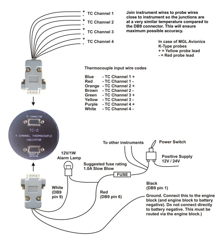
The use of an external 1A fuse is recommended. Connect the supply terminals to your aircrafts power supply. The TC-2 can be used on both 12V and 24V without the use of any pre-regulators. Ensure that the supply voltage will not drop below 8V during operation as this may result in incorrect readings.
