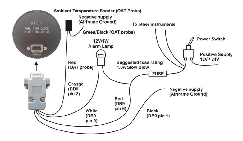
The use of an external 1A fuse is recommended. Connect the supply terminals to your aircrafts power supply. The RTC-1 can be used on both 12V and 24V without the use of any pre-regulators. Ensure that the supply voltage will not drop below 8V during operation as this may result in incorrect temperature readings.
