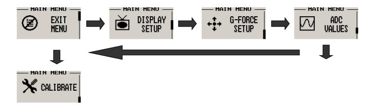
**Note:** (ADC Values and Calibrate Menus are only visible when powering up the unit and pressing the Rotary Control). The text "CALIBRATE" will appear on the intro screen when entering this mode.
