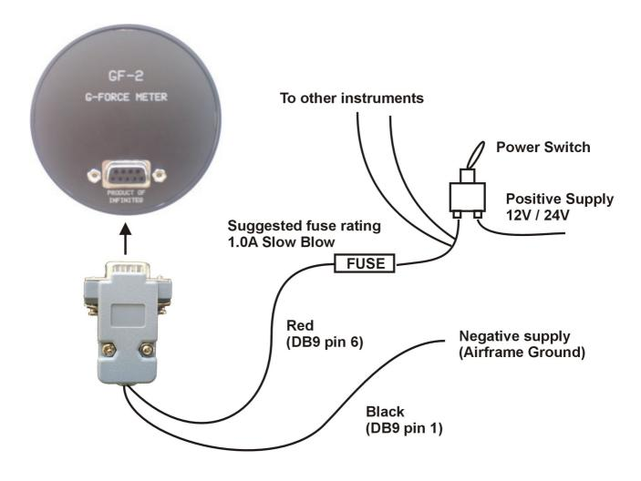
The use of an external 1A fuse is recommended. Connect the supply terminals to your aircrafts power supply. The GF-2 can be used on both 12V and 24V without the use of any pre-regulators. Ensure that the supply voltage will not drop below 8V during operation as this may result in incorrect G-force readings.
