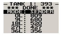
The fuel level sender needs to be calibrated before it can be used with this system. The calibration allows the system to learn the shape of your tank as well as any errors your fuel level sender or installation has.
