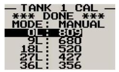
You may want to set individual calibration points manually. For example you may find that your fuel level is over reading at a specific fuel level. Correcting the tank level reading for this area can be simply done by adjusting the calibration point. You can do this by moving the float level with your hands to the desired position and then performing the calibration as outlined above, or you can use the manual option.
