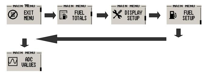
**Note:** ("ADC Values" menu item is only visible when powering up the unit and pressing the rotary control). The text "CALIBRATE" will appear on the intro screen when entering this mode.
