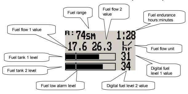
3.3 Single fuel flow and dual fuel level senders (dual tank)
