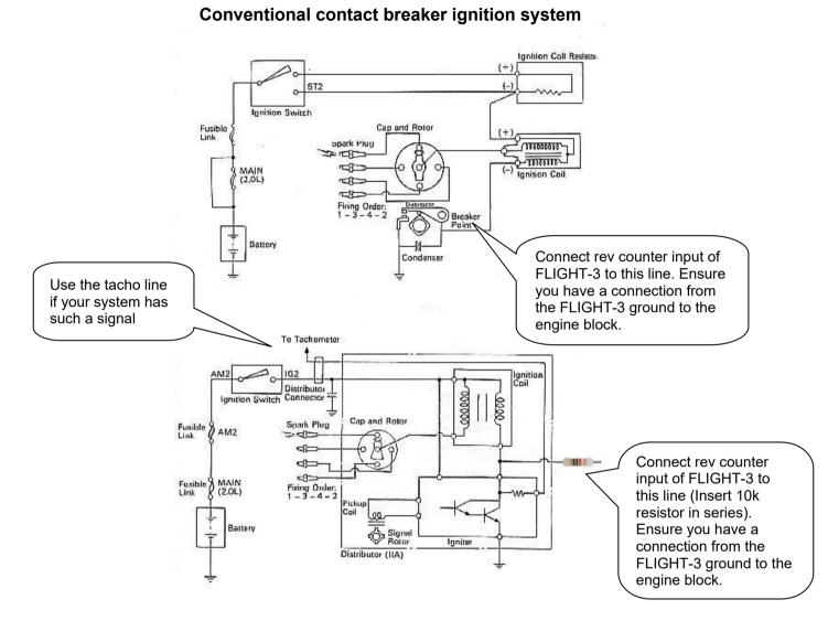
Electronic ignition system with conventional ignition coil
