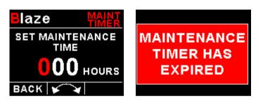
This function allows you to set an engine maintenance timer. This timer is set in engine hours and it will count down to zero when the engine RPM is greater then the *"HOBBS RPM"*. A good use for this function is to set the hours until your next spark plug change or engine inspection. Use the rotary control to change the value.
