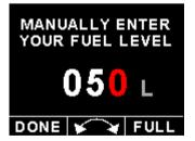
Press the F1 key during the main display screen to manually enter your current fuel level after fueling or defueling your aircraft. This function is only available if you have selected fuel level is calculated from fuel flow. Press the F2 key as a "quick fill button" to the full level.
