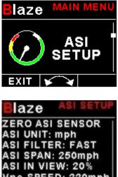
ASI SPAN: 250mph ASI IN VIEW: 20% Vne SPEED: 220mph Vno SPEED: 180mph Vfe SPEED: 50mph Vs1 SPEED: 30mph Vs0 SPEED: 20mph Vs0 SPEED: 20mph Vs ALARM: ON Vne ALARM: ON CAL: 100% 77mph BACK
