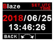
This function is used to set the internal real time clock. The time to be entered must be UTC in order for the system to operate correctly. Do not enter local time (unless it is the same as UTC).
