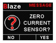
Select this function to indicate to the FLIGHT-3 that zero current is flowing through the MGL Avionics Closed Loop Current sensor. This is best done with the MGL Closed Loop Current sensor disconnected from the main current supplying conductor.
