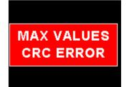
Max Values CRC error. Load default settings to restore to factory defaults. If the error message still persists then it could possibly be a non-volatile memory failure in which case the instrument will then have to be returned to the factory.
