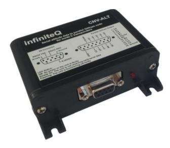
The CNV-ALT accepts RS232 serial data from a compatible MGL Avionics instrument and produces parallel Gillham codes in a format compatible with mode C transponders. The ASV-2 serial protocol must be set to MGL Avionics.
