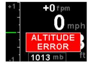
Altitude sensor error. The instrument could have a faulty altitude sensor in which case the instrument will then have to be returned to the factory.
