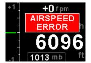
Airspeed sensor error. The instrument could have a faulty airspeed sensor in which case the instrument will then have to be returned to the factory. (Digital airspeed sensor models only)
