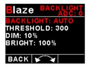
Allow 3 seconds for the display to adjust to the ambient lighting conditions when using the automatic backlight mode. The display will set the backlight to the dim setting if the ambient light is less then the threshold setting, alternatively the display will set the backlight to the bright setting if the ambient light is greater then the threshold setting. The ambient light received is shown as the ADC value in the top header. Use this value to set the threshold value.
