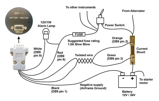
The use of an external 1A fuse is recommended. Connect the supply terminals to your aircrafts power supply. The BAT-1 can be used on both 12V and 24V without the use of any pre-regulators. Ensure that the supply voltage will not drop below 8V during operation as this may result in incorrect voltage and/or current readings.
