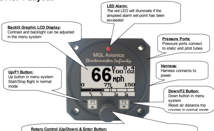
Press the rotary control during normal mode to access the menu system. Rotate anti/clockwise for up/down menu scrolling. During normal mode rotating the rotary control
