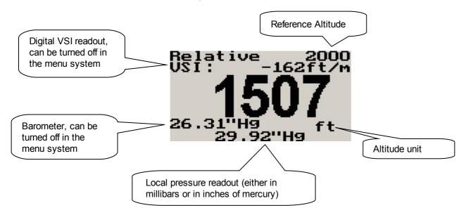
Use the rotary control to adjust the local pressure setting. Pressing the F1/up key will allow the pilot to enter a reference altitude.
