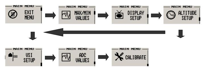
**Note:** (ADC Values and Calibrate Menus are only visible when powering up the unit and pressing the Rotary Control). The text "CALIBRATE" will appear on the intro screen when entering this mode.
