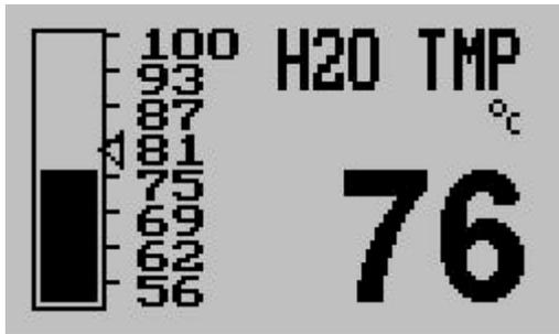
Coolant temperature, usually water temperature of your water cooled engine.
