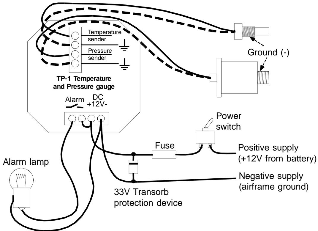
Connect the supply terminals to your aircraft's power supply (you need a dropping resistor or pre-regulator for 24/28V systems).
