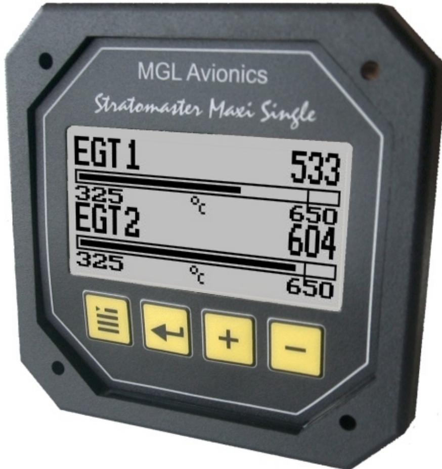
The TC-2 thermocouple temperature display unit is a 3.5" instrument that can be configured to perform the functions of a single, dual, triple or quad channel temperature indicator. Typical uses include EGT or CHT gauges. Each channel displayed can be setup independently for temperature ranges as well as alarms. The instrument is fully programmable by the user resulting in the most flexible solution available.
