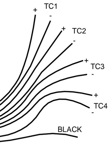
Join instrument wires to probe wires close to instrument so the junctions are at a very similar temperature compared to the D-15 connector. This will ensure maximum possible accuracy.
