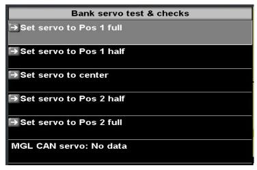
Use the provided functions to move the servo arm to the positions provided. Ensure that servo movement is smooth and no danger exists that could result in binding controls or jamming of control surfaces.
