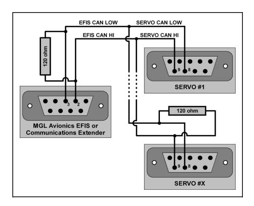
Please note that CAN requires termination resistors to be fitted to the ends of a cable run and that any branches from the cable must be short stubs.
