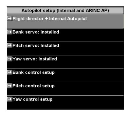
Select each servo that you have installed to gain the relevant setup menu for that servo.
