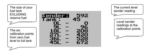
Performing the calibration procedure. Note: You start with an empty tank, you need a measuring jug or fueling device that has calibration marks and you need enough fuel to fully fill the tanl.
