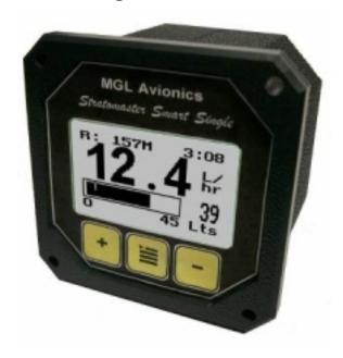
The FF-1 fuel management computer is a 2.25" instrument intended for efficient monitoring of fuel related information onboard small aircraft.
