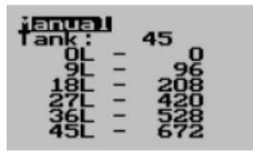
When you are in manual mode, use the "+" and "-" keys as before to select the point you want to calibrate. Then press the Menu key. This allows you to change the value at the calibration point using the "+" and '-' keys. When you are done, press the Menu key again. To end the calibration, move the highlight past the last calibration point as before.
