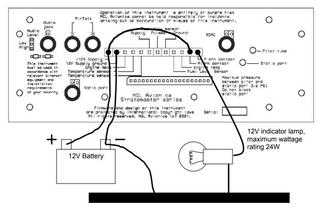
Please note: The drawing above leaves out the switch between the (+) terminal of the battery and the *Stratomaster E2* unit for the sake of clarity.
