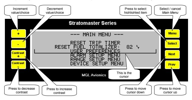
A menu consists of a list of *menu items* with the currently selected item being highlighted by the socalled *cursor*. The *cursor* may be moved up and down through the list using the **NEXT** and **PREV**  keys. In some cases there may be more items than can be displayed on one screen. In this case, selecting **NEXT** (at the bottom) or **PREV** will scroll the entire display to reveal the hidden items. To select or activate the highlighted entry, press the **SELECT** key.
