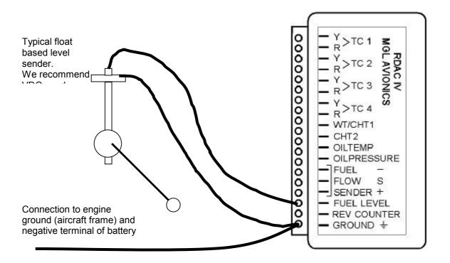
The *Stratomaster RDAC* permits the connection of a standard automotive fuel level sender. These senders can be obtained at automotive spares outlets at reasonable cost.
