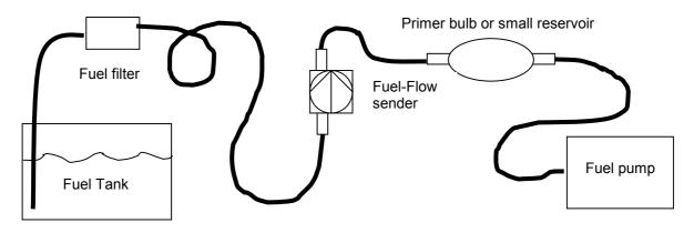
As indicated in the recommended fuel flow sender installation drawing, it can be of advantage to install the flow sender in such a fashion that the inlet points down and the outlet points up. This prevents vapour from forming a bubble inside the flow sender.
