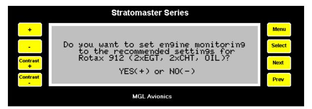
After selecting the required engine, we must confirm the operation by pressing +. Pressing any other key cancels the operation.
