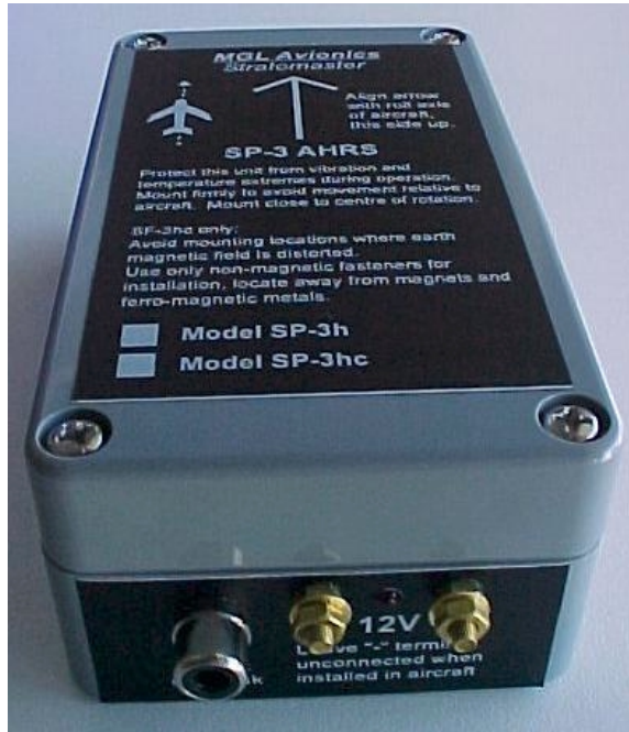
Photo of the SP-3 unit installed in a non-magnetic IP-65 class housing, showing data connector and power supply terminals.
