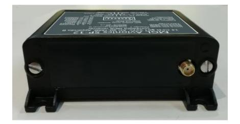
The SP-12 provides a SMA type antenna port at the rear of the SP-12 housing. The SP-12 is designed to support only active GPS antennas that have a supply voltage range from 3.0 to 3.3V DC. Most active GPS antennas on the market today would be compatible with this requirement. The SP-12 is not intended to be used with passive GPS antennas.
