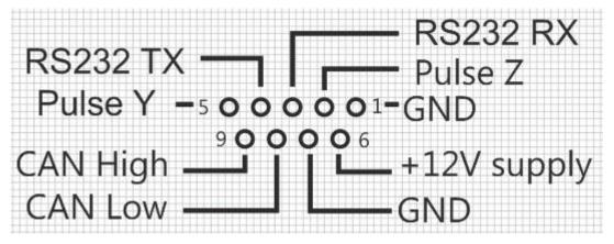
Pinout of the connector of the SP-12. If you are wiring up a male counterpart, this layout is applicable to the view on the solder or cable side of the connector.
