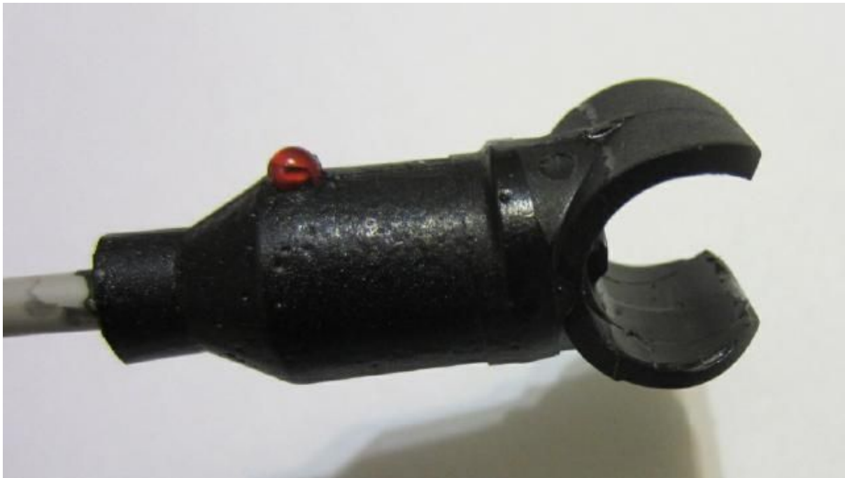
Image of the moulded sensor body. It clips onto the sensor body. The body contains the sensor and a small micro processor used to linearise the flow reading derived from the vortex suspended rotating object in the sensor housing.
