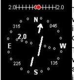
This image shows the two types of GPS based CDI displays supported with the current version of the EFIS. The top display is a true CDI which in this case is telling you that you are about 2 miles to the left of the desired track and you should steer right to intercept the track.
