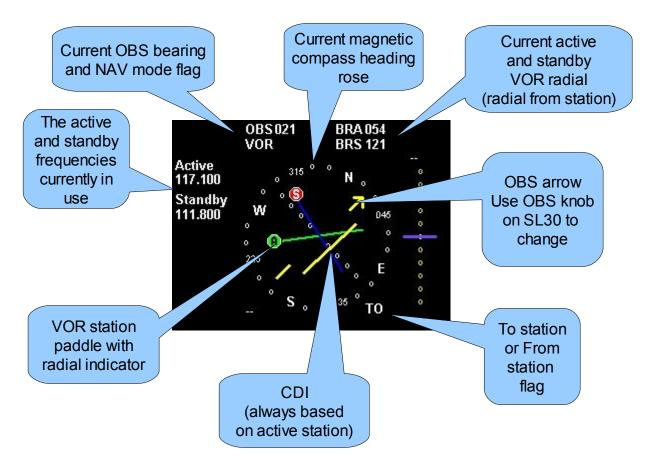
The OBS knob on the SL30 radio is used to set the OBS arrow to the desired radial of the active VOR station. The CDI indicator shows you if you have intercepted the radial – this occurs if the CDI is centered with the OBS arrow. If you maintain a centered needle the needle will point up (you are moving towards the station on the selected OBS radial) or down (you are moving away from the station on the selected radial).
