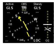
Example HSI and GSI display during a GLS approach onto a runway. The OBS has been set automatically as the runway heading is known. This display shows us that we are slightly to the left of the centerline while crabbing to the right. We are also a little below the glide slope.
