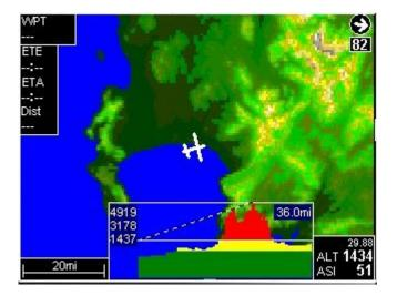
In the absence of raster image maps, the EFIS can use terrain data to create topographical maps using shades of color to indicate ground elevation. A typical image this creates is shown above of the Cape Town area, where your EFIS instrument has been developed. No particular setup is required. If your SD does not contain any raster map data for the area under consideration but terrain data is available, the terrain data will be used automatically.
