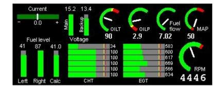
Engine area, here showing a typical 6 cylinder setup with two fuel tanks
