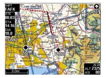
On the moving map the current route leg and next leg (if applicable) are shown as bold red, dotted line. The above image shows a typical view. We have a route leg from FASH to Fisantekraal with the next leg in the route slightly north of west.
