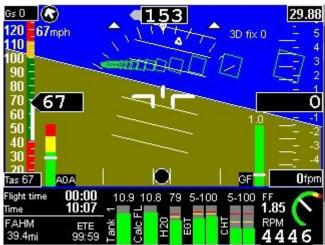
This image shows a typical Highway in the sky (HITS) display. The desired flight path should go directly through the center of the green boxes. In this image, the aircraft is to the left of the desired track and too low. We can also see that at the current heading, we will be intercepting the track soon but we should also climb to intercept the desired altitude.
