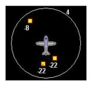
Traffic is displayed as a small yellow square with red border and can be trailed by a red flight path if previous history of this intruder is available. Underneath the intruder the relative altitude is displayed in steps of 100 ft. Negative values mean the intruder is below your altitude while positive numbers show intruders above your flight altitude.
