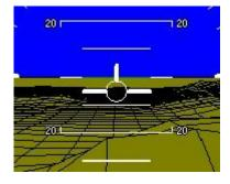
Velocity vector showing a descent at a 5 degree angle
