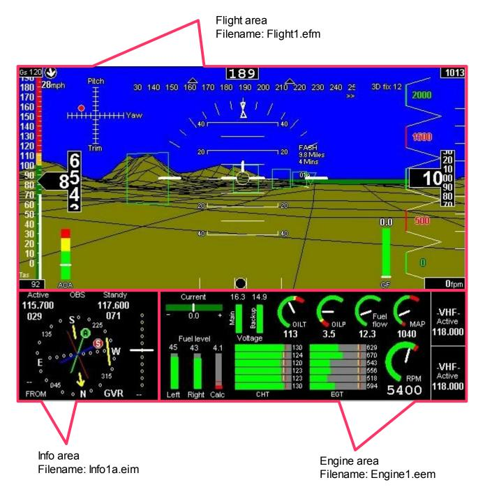
Copying screen designs from one of the 9 possible screens to another is a simple matter of renaming the screen files. For example, to copy the engine part of the above screen to screen number 5, copy the file Engine1.eem to Engine5.eem.
