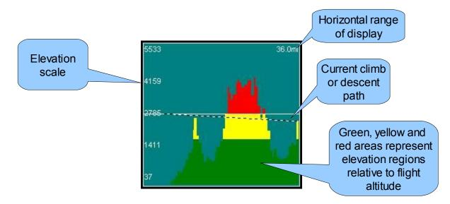
Ground elevation at or above your current flight altitude is shown in red. The elevation from your current flight altitude to 1000 feet (300 meters) below it is shown in yellow.
