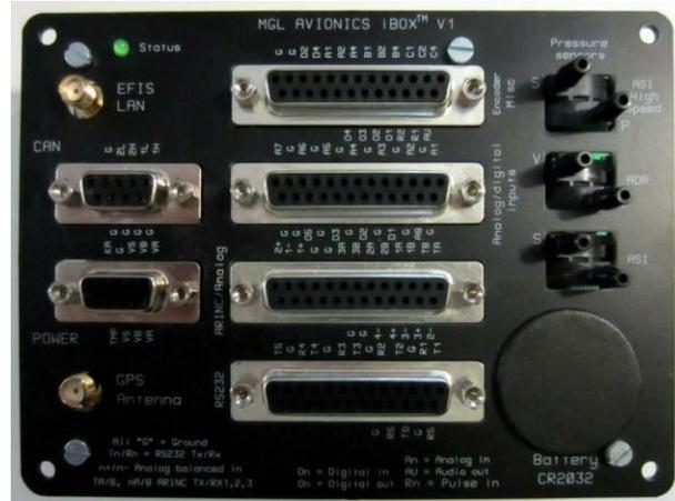
Either one or two iBOX systems can be installed in a single system. One of the iBOX units is the “master”. A second iBOX is a “hot standby”. All external devices are wired to both iBOX units. The “Hot standby” is passive, not taking part in any control or outputs to external devices. On pilot demand or by automatic switchover, the “hot standby” can take full control from the “master” iBOX. In this case the master iBOX will disconnect its outputs.
