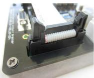
Image showing connector with strain relief clip inserted in one of the ECB connectors. The two restraining clips clip over the strain relief and hold the connector securely in place. To remove the connector, simply force the two clips apart - this levers the connector out.
