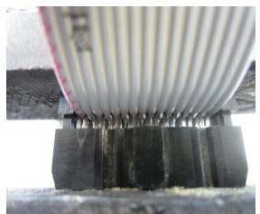
Close-up of the connector before closing it using the vice. Note how each cable core lines up exactly with its corresponding connector blade.
