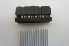
A small triangle on the connector denotes "pin 1". It is not of importance in this application. You can insert the cable from either side of the connector as you wish.
