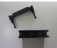
Image showing the cable strain relief clip.
