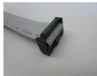
Fold the cable over the top of the connector and insert the train relief clip until it latches on both sides.
