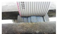
Image showing the connector closed. Only a small force is needed when using a bench vice.
