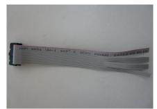
Image of a short cable connection ready for use. Split off 4 groups of 4 wires as shown in the image. There is no practical restriction to the length of the cable, you can make it any length you need. The ECB kit contains about 10 feet of 16 way ribbon cable. Contact your supplier if you need longer cable.
