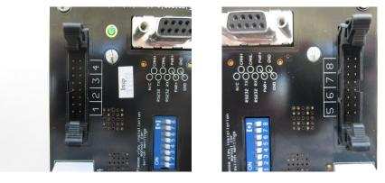
Each connector serves 4 breakers using 4 conductors:
