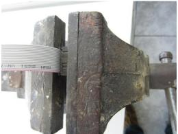
Insert the cable so a few mm shows on the other side. Ensure cable is straight and the connector blades line up exactly with each cable core. Then simply use the vice to squeeze the two connector parts together until they latch.
