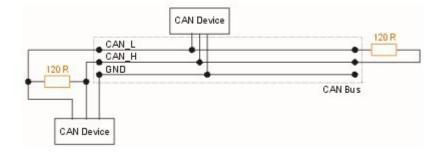
The connection uses two wires which are twisted around each other. This forms a "balanced transmission line". It helps to reduce emissions and also makes the link more robust against external interferences.
