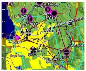
Note that one of the waypoints in the route is highlighted with a white background? We can move that highlight using the up and down arrows. This is the waypoint that will be used for insert, delete, edit and other modes.
