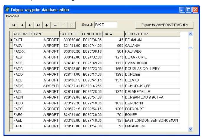
Each waypoint has a data record. The use of this depends on the waypoint type. For airports, this is the elevation (currently fixed in feet). For navaids, this is the frequency in Mhz. Intersections have the value 0 (the data is not used for anything).
