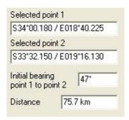
Flight planner contains an easy to use distance and bearing calculator that works right from the map. Click on any two locations and select "select this point". Flight planner will give you a very accurate result regardless of distance as Flight Planner takes the exact curvature of the Earth into account (using WGS84 survey data).
