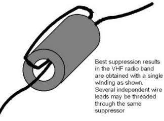
It is permissible to thread several wires through a single ferrite.
