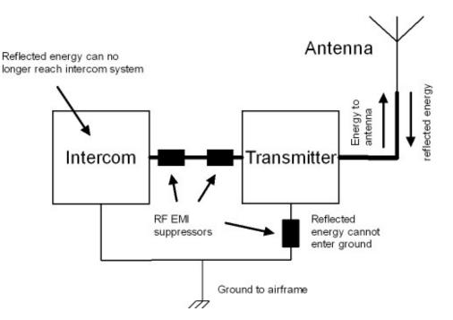
In this case three ferrites are employed. Two are placed on the audio cables to the transmitter, one on each end, about 5 cm (two inches) from the ends of the cables.
