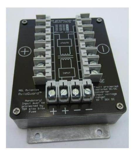
Fault protected, wide input range, isolated, DC to DC converter for avionics applications
