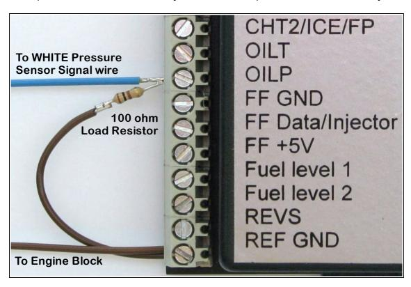
Example installation: 100 ohm load resistor fitted to RDAC VD
