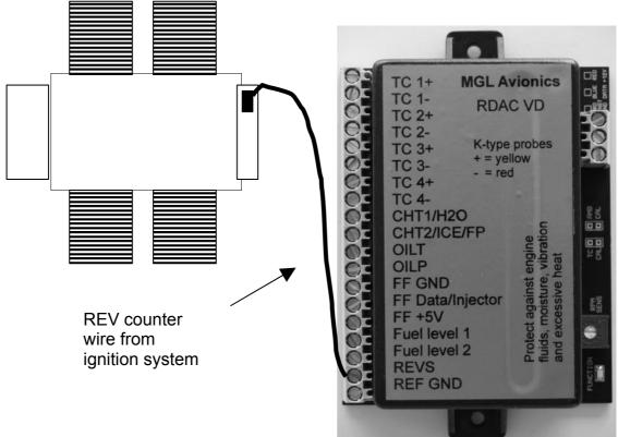
After you have connected the rev counter terminal to the signal source you need to set the number of pulses per 10 revolutions in the Calibration Menu. The calibration itself depends on your engine type and what kind of signal you are using. Typical sources are:
