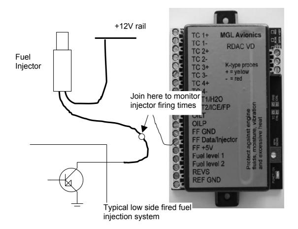
Should you want to monitor fuel flow directly by means of measuring the fuel injector opening time, the above arrangement can be used. You can use both high or low fired injectors (most systems are low side fired as shown above).
