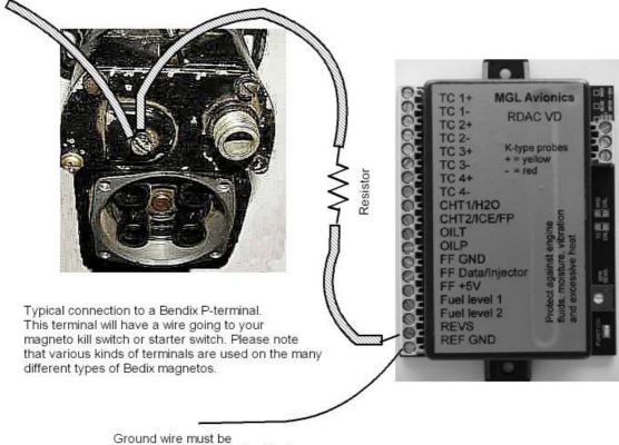
connected to your engine block. Engine block must be connected to battery minus.
