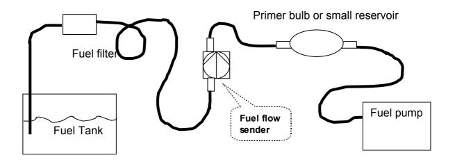
As indicated in the recommended fuel flow sender installation drawing, it can be of advantage to install the flow sender in such a fashion that the inlet points slightly down and the outlet points slightly up. This prevents vapor from forming a bubble inside the flow sender.
