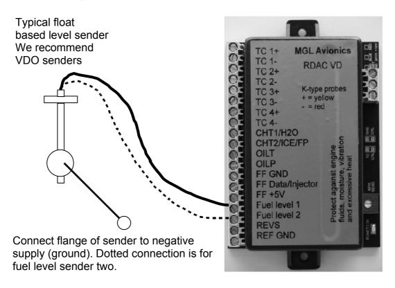
The Stratomaster RDAC VD EMS permits the connection of one or two standard automotive fuel level senders. These senders can be obtained at automotive spares outlets at reasonable cost.
