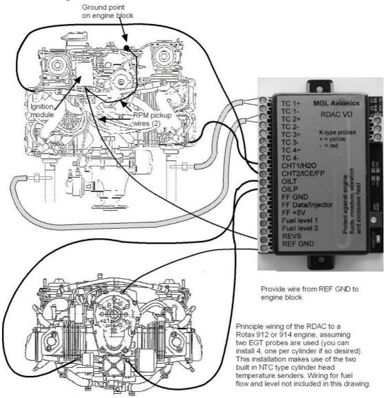
The Rotax 912/914 contains two built in NTC type CHT temperature senders. In addition oil temperature and oil pressure sender is provided as standard. Due to the fact that the 912 has two carburetors (one for each side of the engine), two EGT probes should be connected, one for each exhaust stack. You can connect four EGT probes if you like. You would use TC1 and 3 as one pair and TC2 and 4 as the other pair. Each pair monitors one side of the engine.
