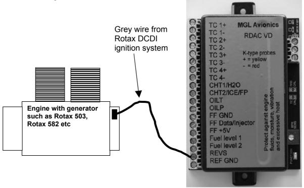
Most instruments assume as a default that you will be connecting a Rotax with DCDI ignition system. Such a system produces 6 pulses for every revolution of the engine.
