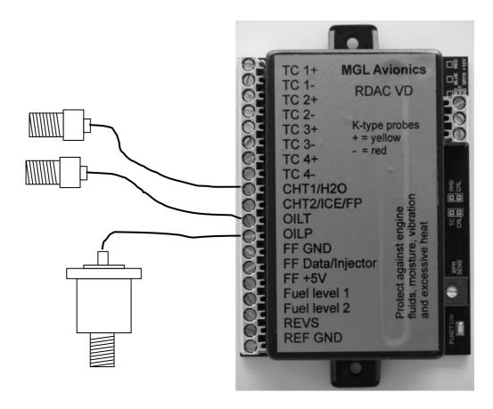
This drawings shows the connection of a coolant temperature probe, a oil temperature probe and a oil pressure sender.
