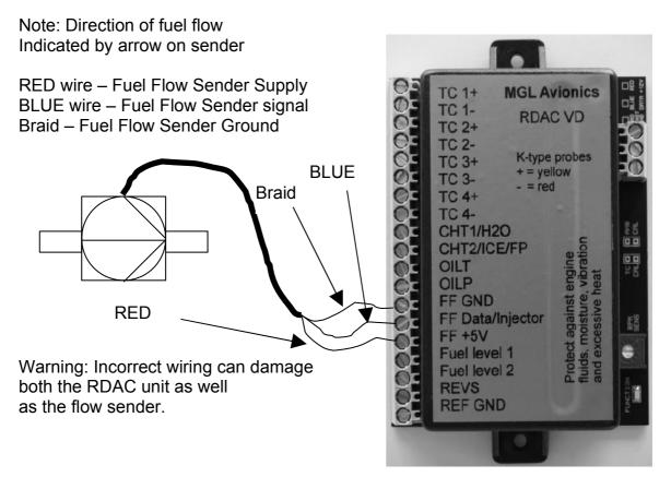
The optional Fuel Flow Sender is highly recommended for use with Stratomaster instruments. It provides instantaneous readouts of hourly fuel usage, and both time and distance estimates on remaining fuel in flight. You can also verify the performance of your fuel pump during the pre-takeoff engine run up – a very valuable check !
