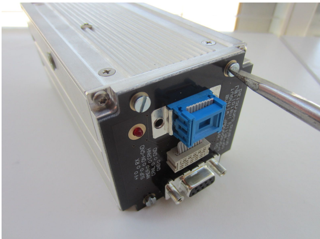
Mount the interface PCB onto the transponder using 4 M3x6 screws. Plug in the blue DB-9 connector into the transponder's socket. Notice the plug has a tight fit.
